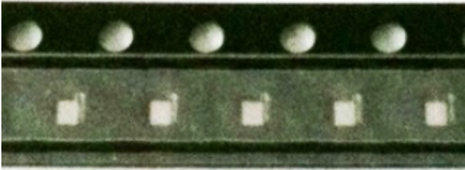
Fig 4. Die on tape and reel
