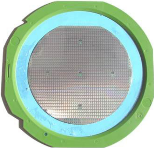
The wafer is sawn.
