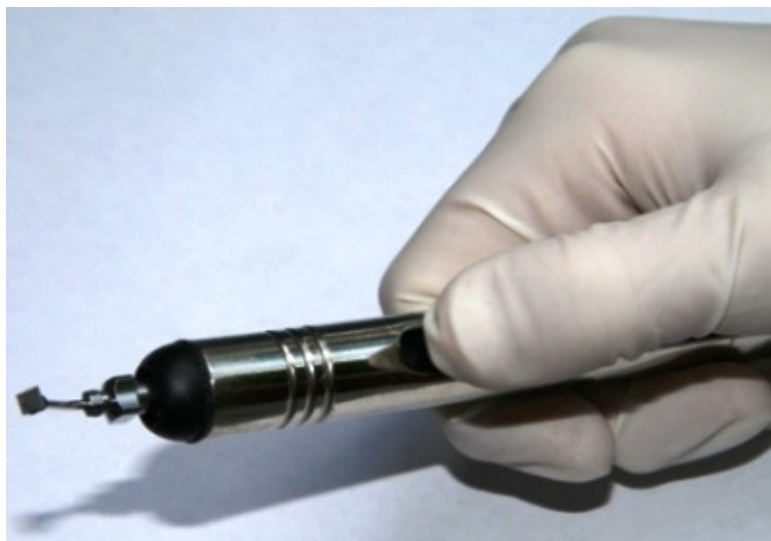
Fig 14. Vacuum pick up tool
